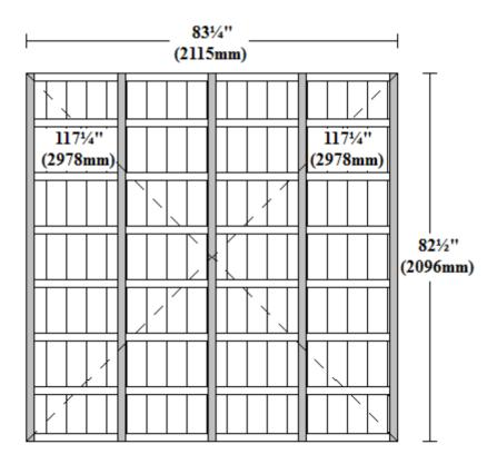
NB:- Floor joists run from left to right. Optional Floor Bearers run from front to back.
